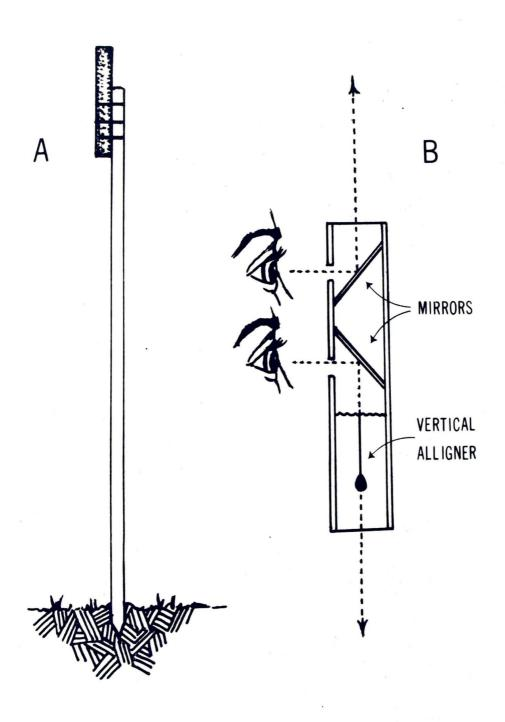
Figure 1. Diagram of the instrument used in detecting presence or absence of foliage in each of three layers above randomly positioned ground points. Drawing A shows the randomly positioned ground points. Drawing B shows a cut-away view inserted into the ground. Drawing B shows a cut-away view of the instrument itself
